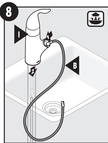
Insert Pullout Hose (B) into opening and feed through
