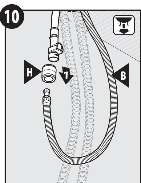
Install Hose Weight (H) onto Pullout Hose (B).
