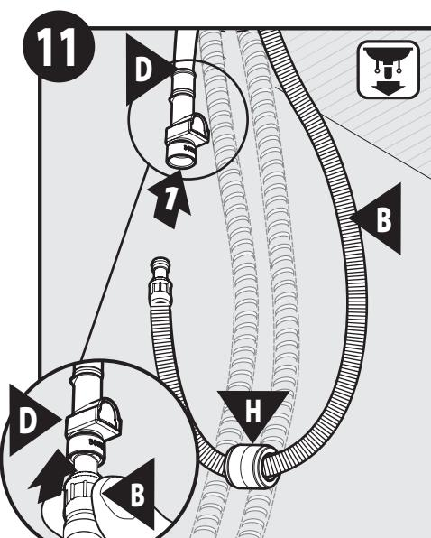
Insert Pullout Hose (B) into Duralock Quick Connect Adapter
