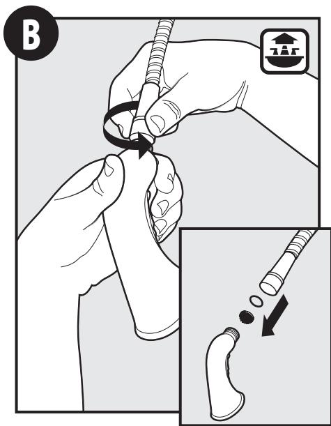
Unscrew Pullout Hose from Spray Wand. Remove Screen & O-Ring.
