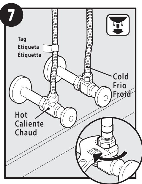
Connect hot and cold supply hoses to water supply valves.
