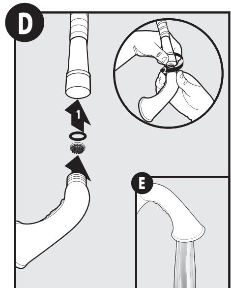
Reinstall Screen & O-Ring as shown. Thread Pullout Hose and Spray Wand. Check water flow.
