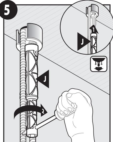
Tighten Mounting Nut with Installation Tool (J).
