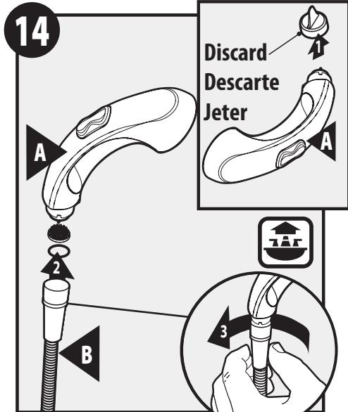
Remove and discard protective cap from Spray Wand (A). Attach Spray Wand (A) to Pullout Hose (B). Finger Tighten.
