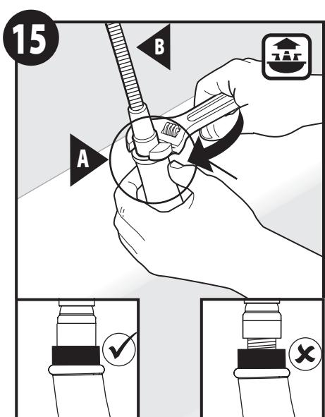
Tighten hose nut with wand. Do not overtighten.
