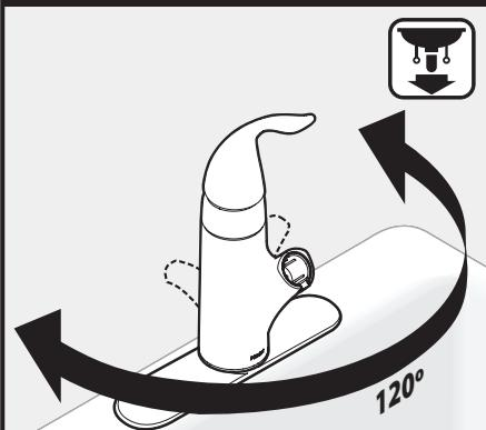
Slide Mounting Bracket (E) onto Faucet Body (I). Secure with Mounting Nut (F).
